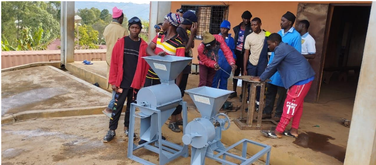
Grinding mill made in the wilding workshop
